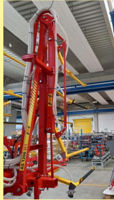
Figure 41: Correct installation of dispersion plate and hose 2
