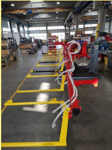
Figure 36: Hose laying along the frame to the outer tine sections
