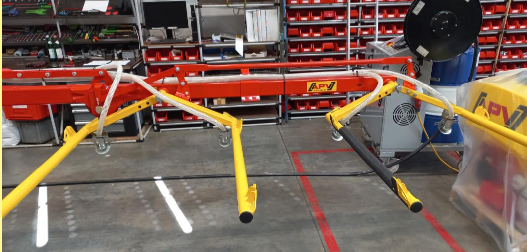
Figure 38: Hose laying to the two outermost tine sections
