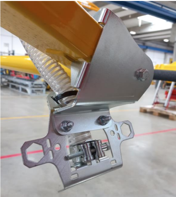
Figure 24: Dispersion plate installation 3 carried out completely
