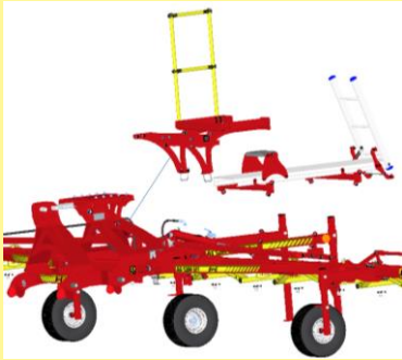
Figure 10: Installation of the platform kit 1
