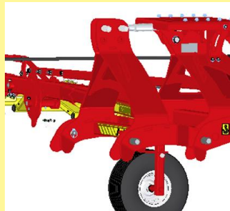
Figure 13: Additional headstock installed
