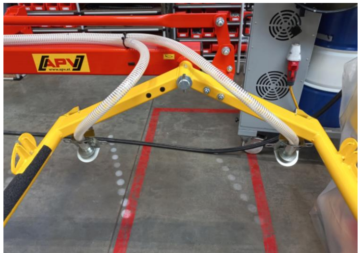
Figure 25: Dispersion plate installation 4 carried out completely
