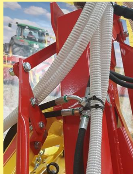
Figure 35: Fastening of the hoses for the scissor folding element
