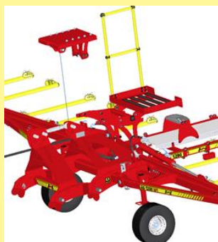
Figure 5: Installation of the PS bracket on the headstock 1
