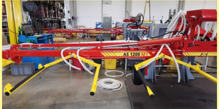
Figure 33: Hose laying over the pivot point of the tine section
