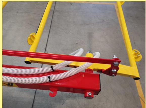
Figure 37: Hose laying over the pivot point of the tine section
