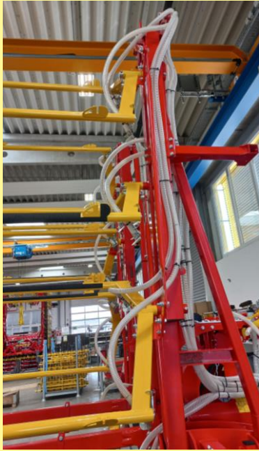
Figure 40: Correct installation of dispersion plate and hose 1
