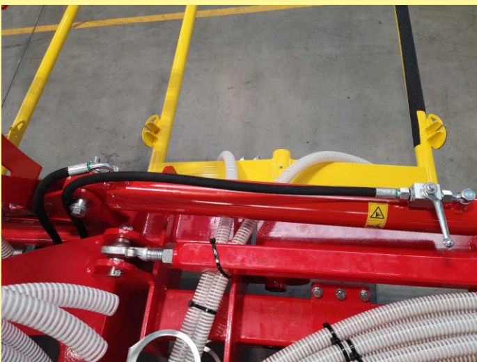
Figure 30: Routing the hoses under the folding cylinder 1
