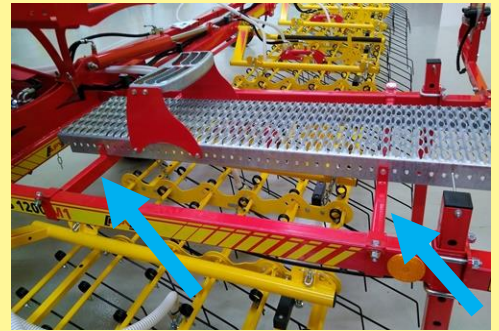
Figure 12: Platform kit installed on the frame of the support stands
