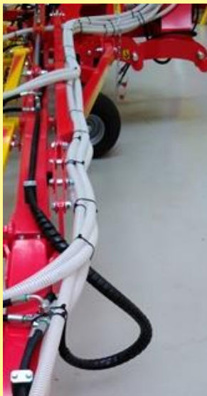
Figure 34: Hose laying along the scissor folding element
