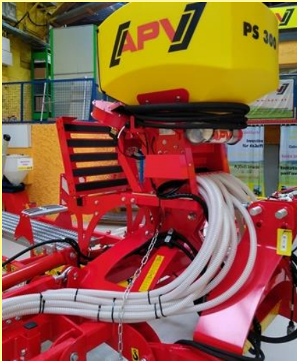
Figure 28: Hose laying starting from the PS on the left side
