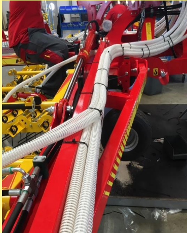
Figure 32: Hose laying along the side frame
