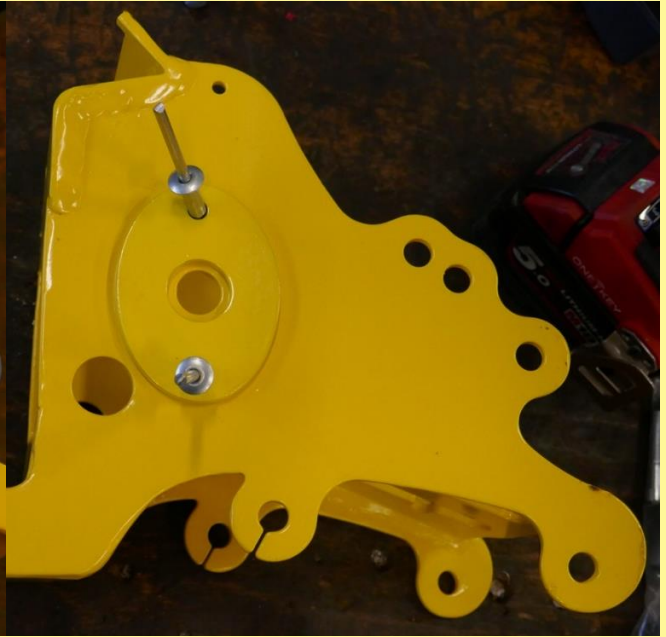
Figure 6: Riveting on the sheet metal profile reinforcement
