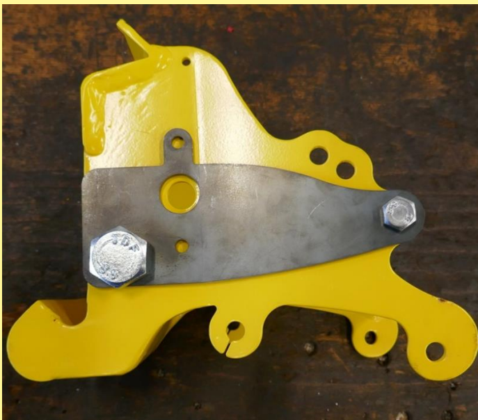
Figure 3: Installed drilling template
