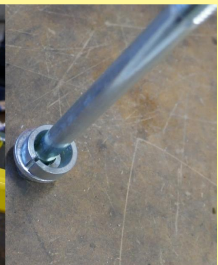
Figure 10: Position of the spring dowel pin
