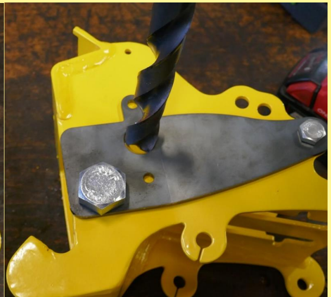
Figure 4: Drilling a 22.5-mm hole
