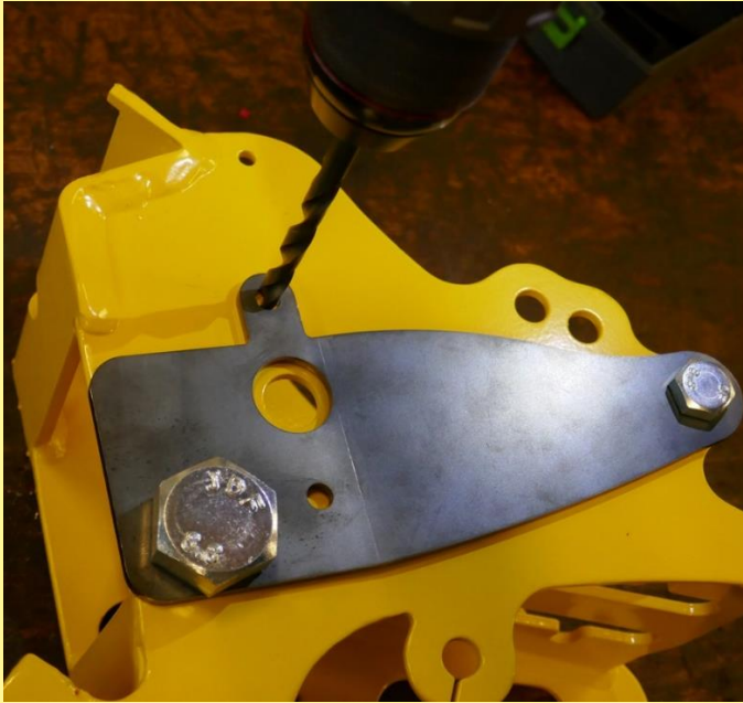
Figure 5: Drilling the 7-mm holes
