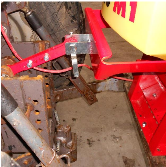
Figure 8: PS mounted on the tractor with three-point mounting bracket 1
