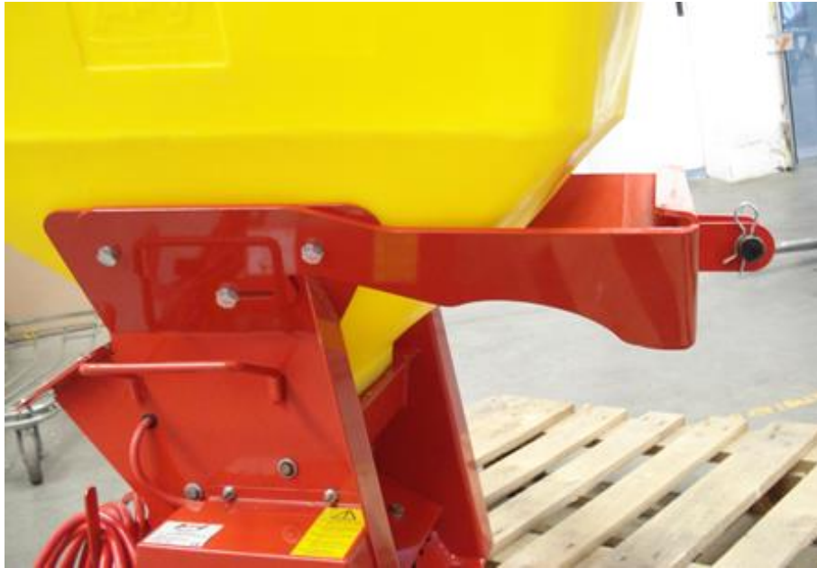
Figure 4: Three-point mounting bracket installed on the seeder 1
