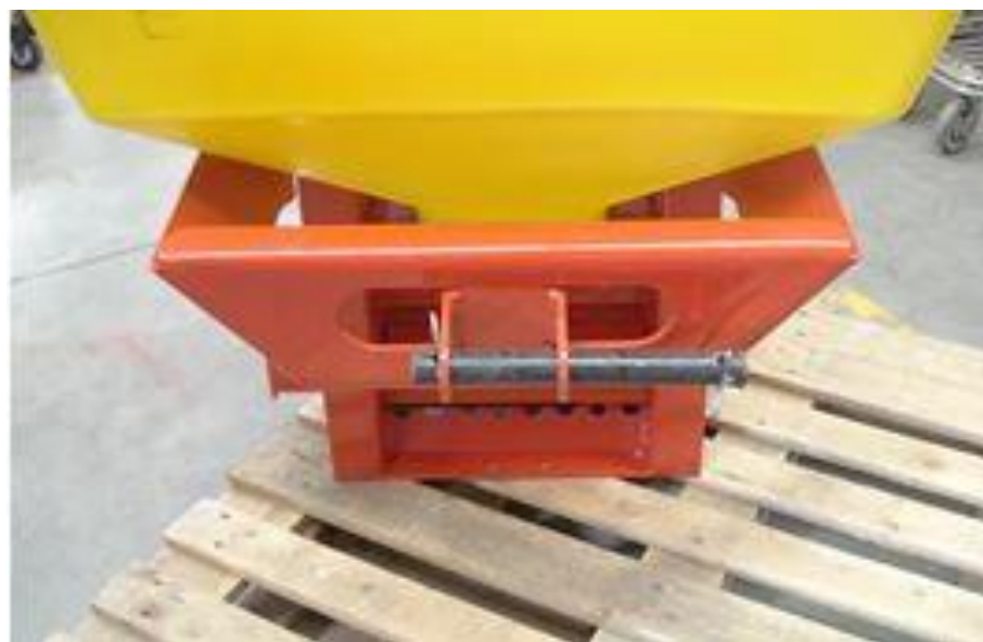
Figure 6: Three-point mounting bracket installed on the seeder 3
