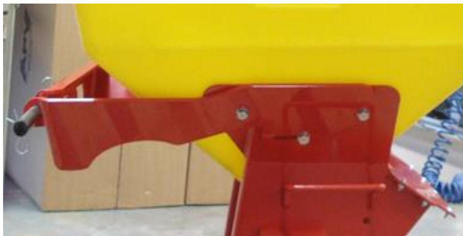
Figure 5: Three-point mounting bracket installed on the seeder 2
