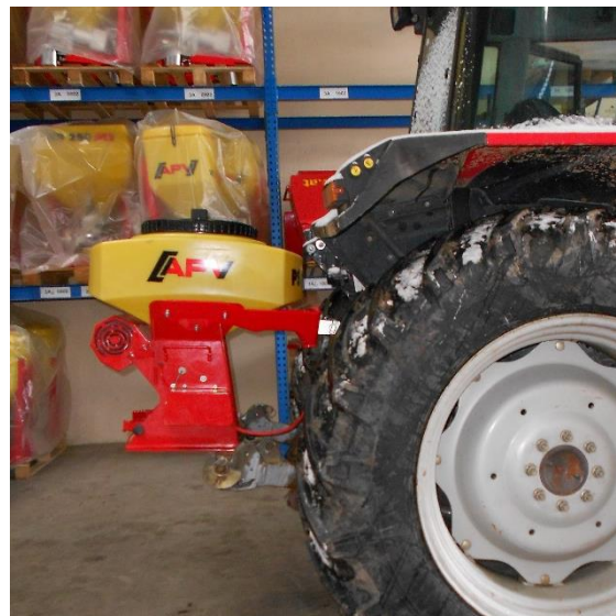
Figure 9: PS mounted on the tractor with three-point mounting bracket 2
